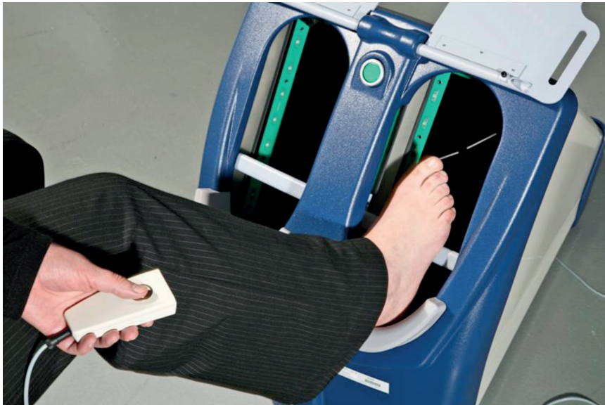
Figure 1. (A) Schematic cross section of the photographic foot imaging device showing the most important features, including (1) camera module, (2) light sources (LEDs), (3) mirror, (4) glass plate, (5) foot supports, (6) lid, and (7) computer. (B) Photograph of the device showing the adjustable foot supports bars and the remote control switch.
